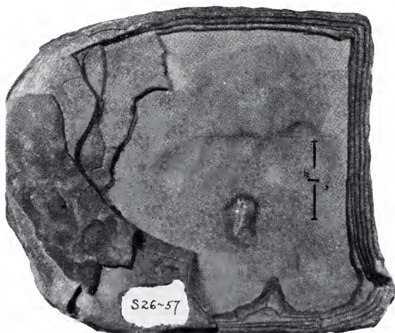
Fig. 3. A partly weathered joint block with rounded edges, showing the gray, unweathered core of fresh rock surrounded by concentric shells of dark, limonitic material which have exfoliated to a considerable degree on the upper side of the specimen. The bedding is in the plane of the page.
